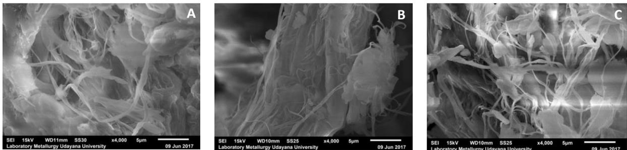
**Figure 2.** The SEM test result with 4000 times enlargement with various SMCs (A=SMC-2; B=SMC-4; and C=SMC-6)
